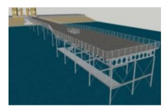
**Stage Three** will be the Pier head construction, a further 120 feet out into the sea, incorporating a fishing/boat platform under the main deck
