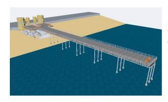
Stage Two will provide the semblance of a pier, with the projection outwards from Stage One. It is envisioned that it will consist of up to 10 identical 40 foot sections. This will ensure that the end of the pier will be in the sea, even at low tide.
